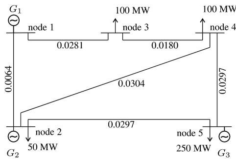
Figure 12: Power system diagram. The numbers close to the lines are reactances in per unit. Source: [11]
