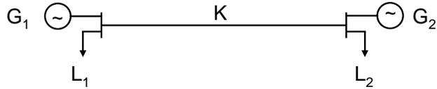
Figure 9: Two bus network with constrained transmission capacity
