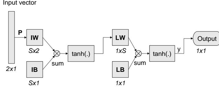
Figure 2: Feed-forward neural network structure
