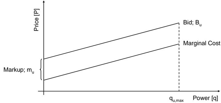
Figure 1: Marginal cost and markup of a generator unit
