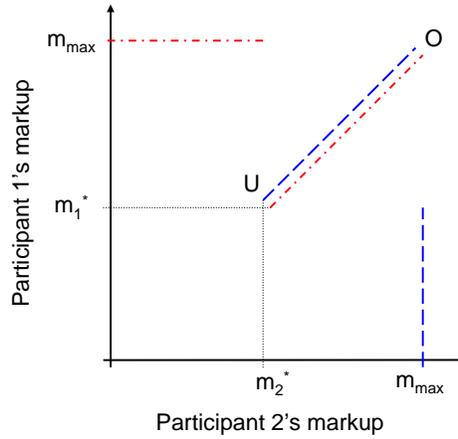
Figure 10: Reaction function of players in the two-bus market, adapted from [19].
